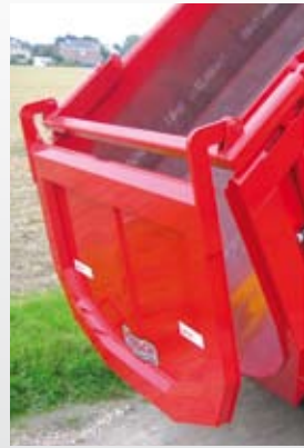
Top-hinged hydraulic tailgate with lock-out feature
