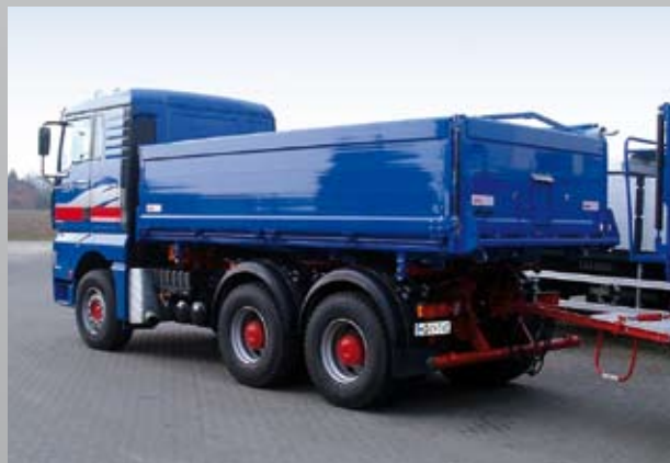
3-way tipper body with split aluminium sidewalls
