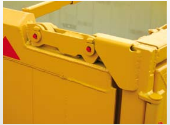
2-way bearing for top-hinged wing-gate frame
