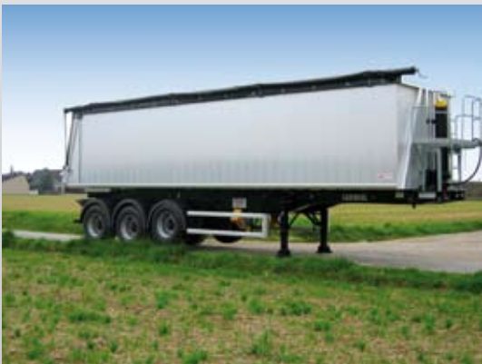
High-capacity bodies made of aluminium
