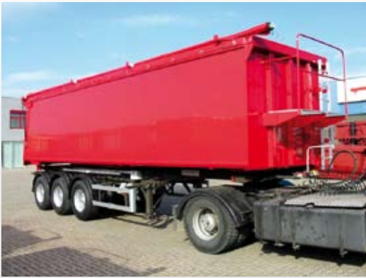
High-capacity bodies made of aluminium
